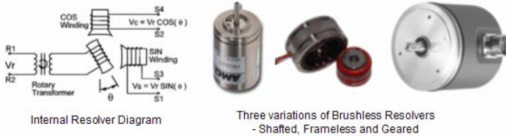
Figure 8. Diagram and examples of resolvers
